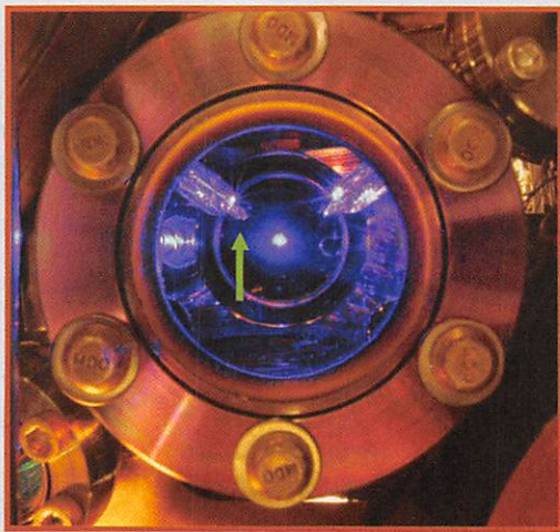
Figure 2. The strontium optical-lattice clock shown here is now the world's most accurate timekeeper. Visible at the center is a cloud of trapped, fluorescing Sr atoms, used to determine the ticking frequency. Key to the clock's accuracy is a temperature sensor (indicated by the green arrow), which is mounted on a retractable glass tube and used to characterize systematic errors caused by blackbody radiation. (Adapted from ref. 2.)
